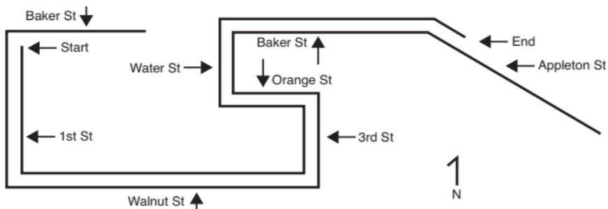
In this example, trying to describe the entire route on one locate request would be very difficult. The excavation site can, however, easily be broken down into individual streets and described as follows:
